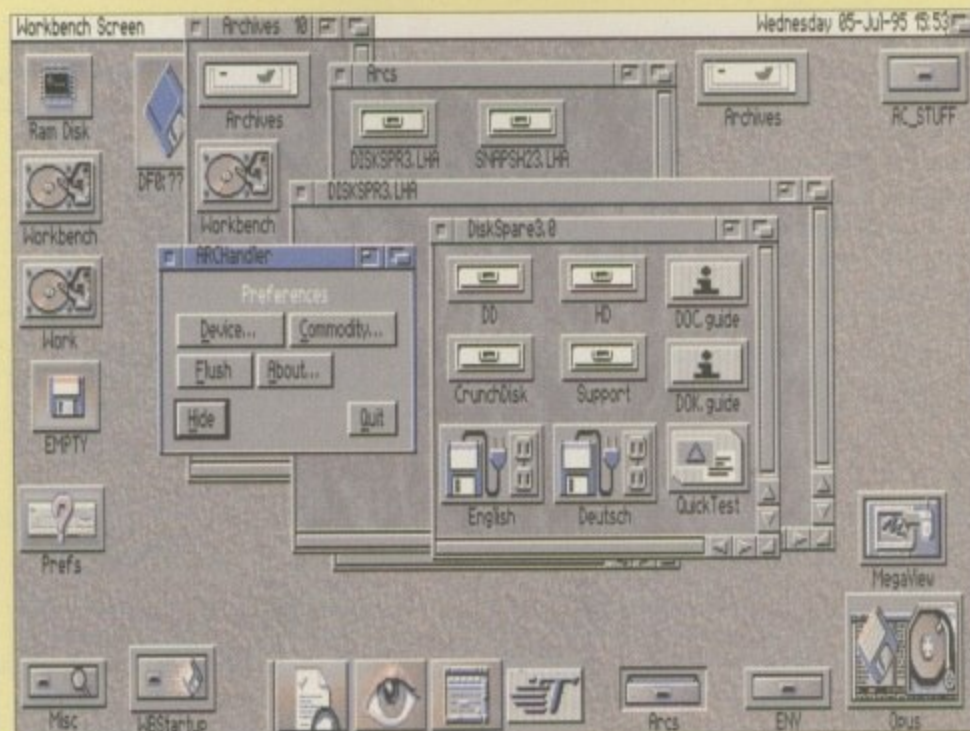
ARCHHandler makes accessing and viewing archived files a breeze by treating the contents as though they were in a normal drawer
